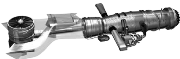
Fig. 3 Shaft-driven lift fan propulsion system.
